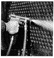
What happens when a tube is totally clogged? Pressure relief valve releases the pressure, protects operator from back-firing brushes when gun is pulled away from tube
