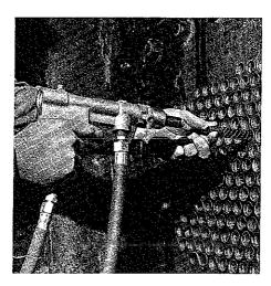
3. Insert nozzle into tube, squeeze trigger. Brush shoots through tube with a spinning, scouring action. Tube is clean—instantly
